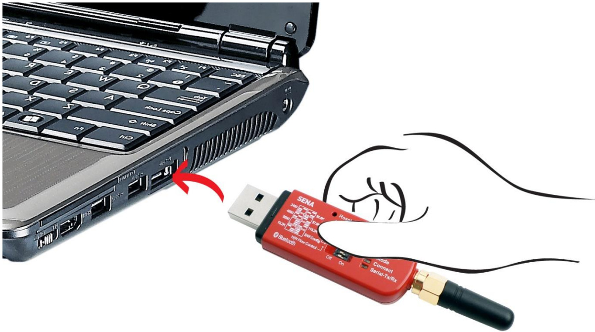
Figure 2-2 Connecting a Serial Device to Parani-SD1000U
